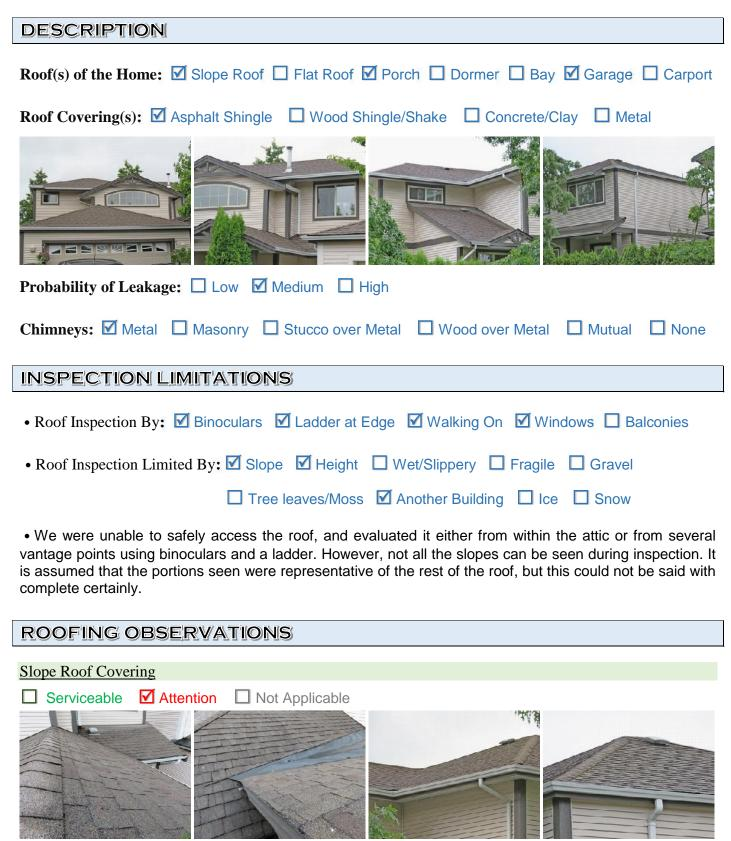
• Moss and/or debris accumulated on the roof at the time of the inspection may damage roof covering materials by retaining moisture. Clearing the roof of debris should be included in annual maintenance.
